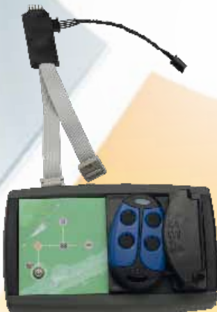
PROGRAMMER TRANSMITTERS - RECEIVER PROGRAMMING DEVICE
